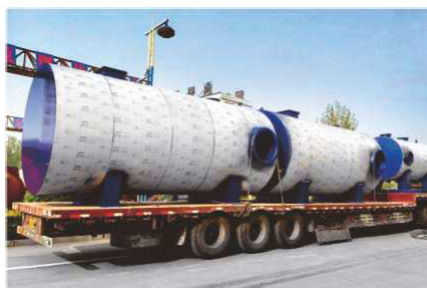
新疆 3台120万大卡热风炉用于烘干棉花 3sets 1,200,000kcal hot air furnaces for Xinjiang cotton drying
