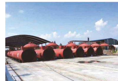
河南太康建材公司 6条31米蒸压釜和8吨冷凝燃气蒸汽锅炉 6 sets 31m autoclaves and 8T condensing gas steam boiler for Henan building materials company
